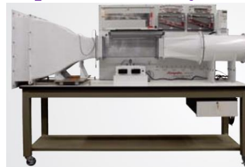
Model H-6910-CDL Wind Tunnel shown with Model H-6910-5 Manometer Package option and Model H-6910-55 Lift and Drag option Dimensions: 69"H x 96"W x 30"D Weight: 1,000 lbs.
